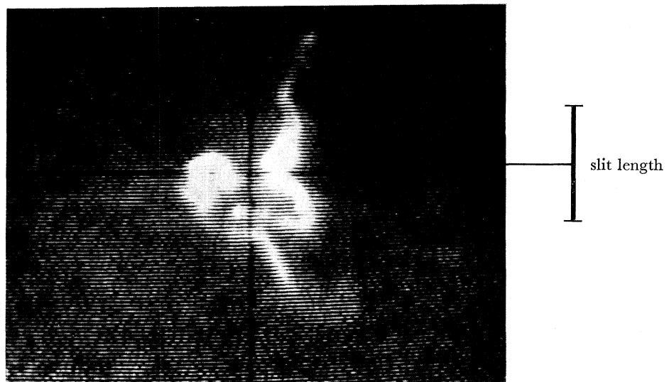
FIGURE 8. Position of the spectrograph slit on the 15 June 1973 flare H \alpha image. The slit was located along the vertical cross-hair.
